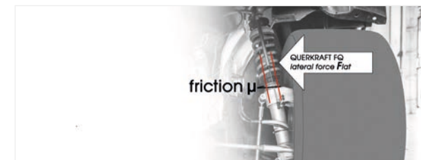
McPherson / friction under lateral force
